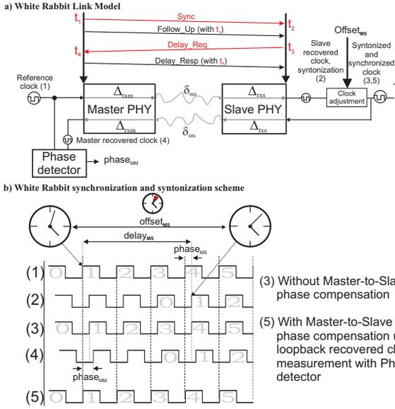
Fig. 3. WR Link Delay Model, synchronization and syntonization scheme.
