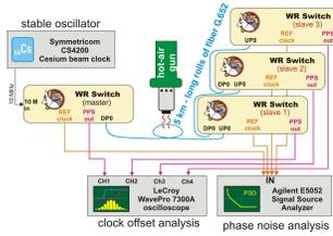
Fig. 7. Test setup.
