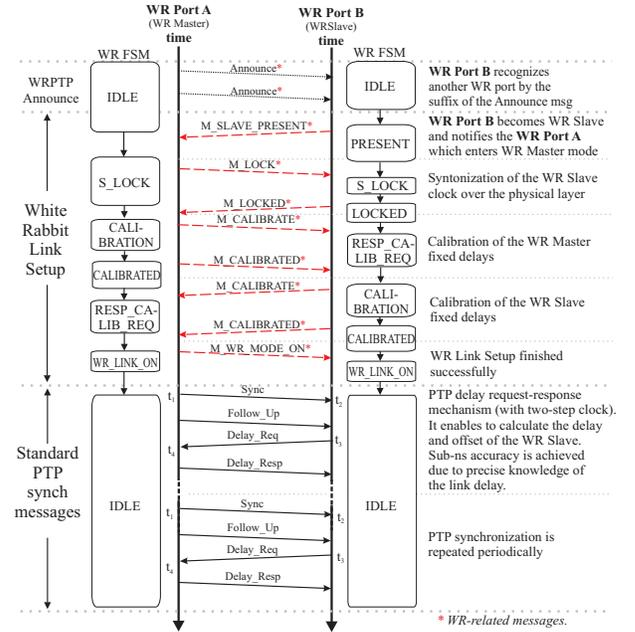
Fig. 2. Simplified overview of the message flow in WRPTP.
