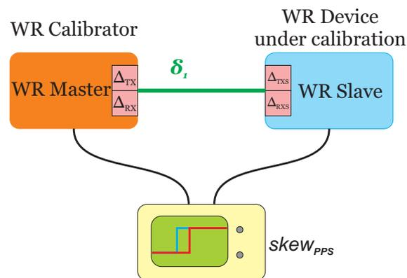
Figure 5: WR Device calibration with WR Calibrator and known fiber  $f_1$
