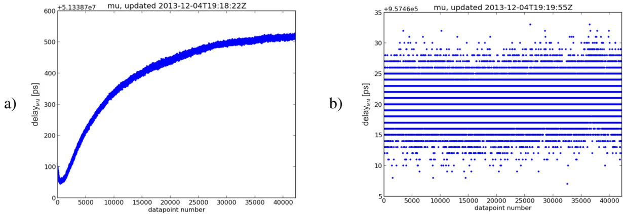
Figure 10:  $delay_{MM}$  of 5 km (a) and 5 m (b) fiber logged for almost 12 hours using two WR Switches
