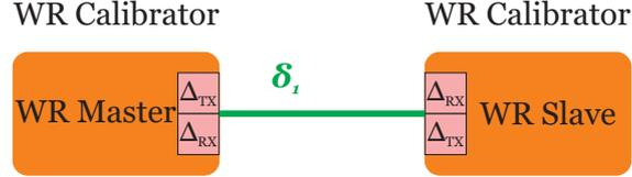
Figure 4: Measuring Calibrator latencies
