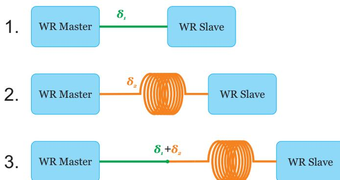
Figure 2: Measuring total fiber propagation latency
