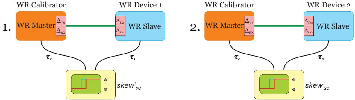
Figure 8: Calibration with 1-PPS delays taken into account
