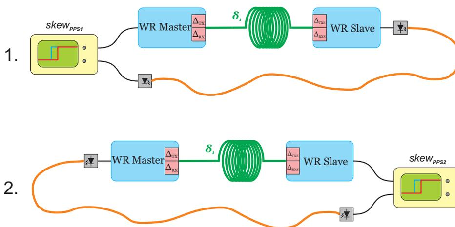
Figure 6: Measuring 1-PPS offset using a loop-back fiber
