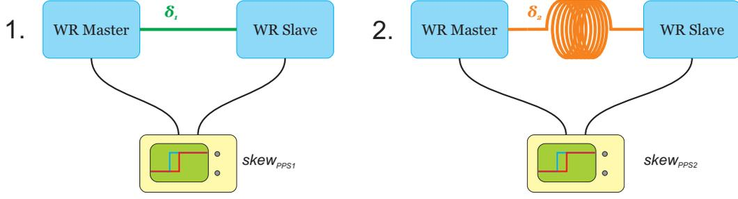
Figure 3: Measuring fiber  $f_2$  asymmetry
