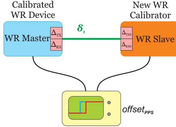
Figure 7: Calibrating a new WR Calibrator for an already-existing WR network
