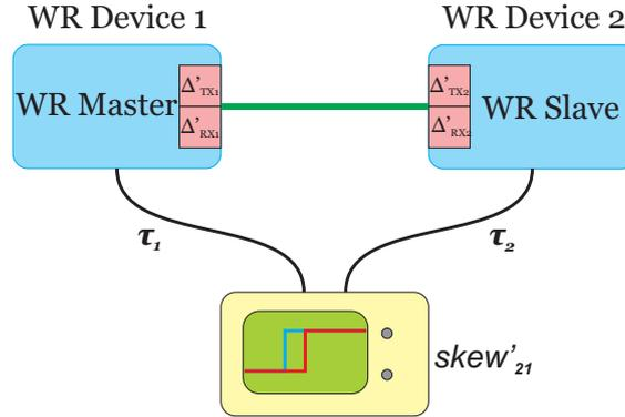
Figure 9: Synchronization of WR Devices calibrated to the same calibrator
